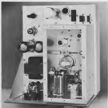
Looking at the top of W2YM's five-band mobile transmitter. Note neutralizing capacitor C_{16} mounted on small bracket and standoff insulation between 6883 and 7054.
